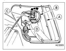
5.8 Remove the front direction indicator light bulbholder by turning it anticlockwise
